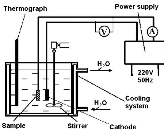
Fig. 1 Schematic view of the micro-plasma oxidation set-up
