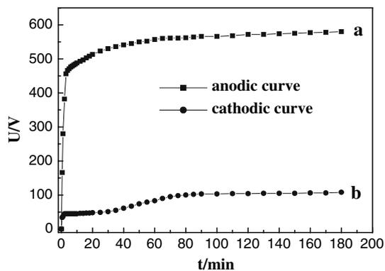
Fig. 2 Voltage–time curve in the micro-plasma oxidation process
