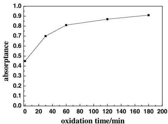
**Fig. 5** The influence of oxidation time on the solar absorptance of the coating
