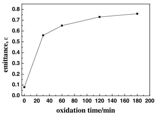
**Fig. 6** The influence of oxidation time on the emittance ( $\epsilon$ ) of the coating
