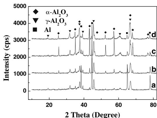
**Fig. 8** XRD patterns of the coatings of different oxidation time (a) 30 min; (b) 60 min; (c) 120 min; (d) 180 min
