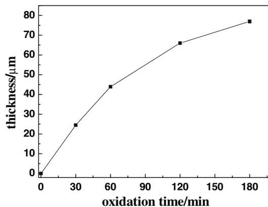
Fig. 3 Influence of oxidation time on the thickness of the coating
