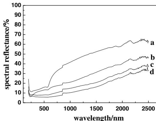
Fig. 4 Influence of oxidation time on the spectral reflectance of the coating (a) 30 min; (b) 60 min; (c) 120 min; (d) 180 min
